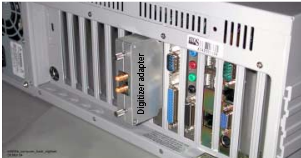
Figure 4 Connect adapter to back of PC digitizer card
